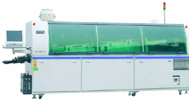
New Lead-free Capable Wave Equipment used at SMT Dynamics
